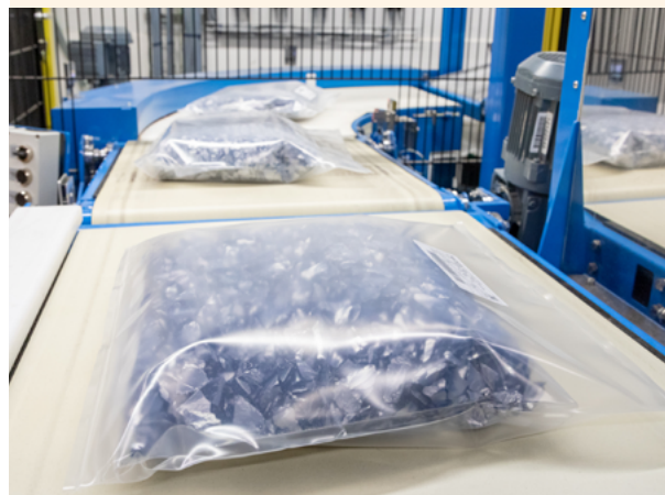
The polysilicon chunks are packaged in plastic film in the cleanroom and then sent to customers.
