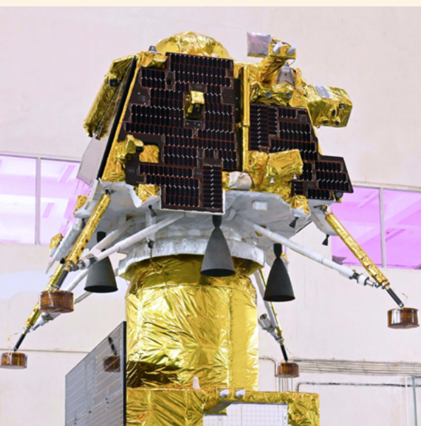
India's Vikram moon lander. Specialty silicones from WACKER are used to bond its solar panels.
